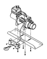
make sure the motor, drum and gearbox housing are aligned correctly.
